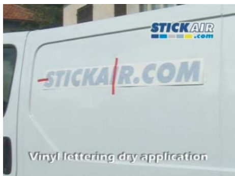
Vinyl lettering dry application Position the lettering where you want it and stick it down using the sticky tape. This will enable you to move your lettering about easily.
