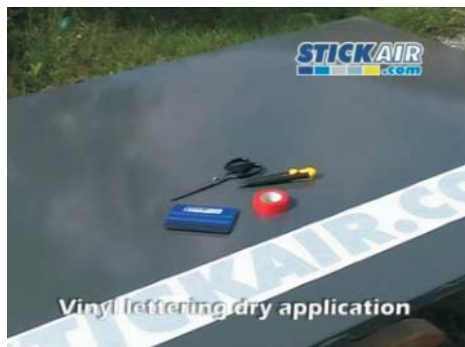
Vinyl lettering dry application For this type of application you will require a few accessories: sticky tape, a squeegee, scissors and a cutter where applicable.
