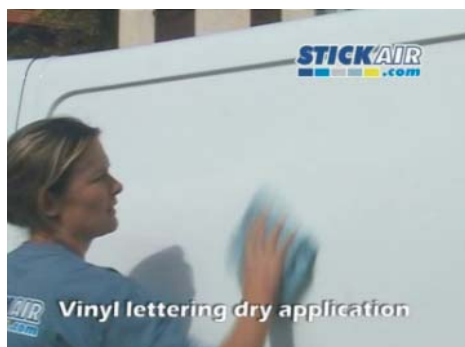
Vinyl lettering dry application Before application it is important to remove any grease from the surface, e.g. using window cleaner.
