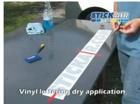
Vinyl lettering dry application Apply a tape tab to the centre of the lettering ensuring that it overhangs each side generously. Also apply a tape tab to one end.
