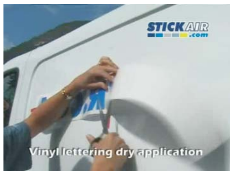
Vinyl lettering dry application Cut the piece of silicon-coated paper using the scissors.
