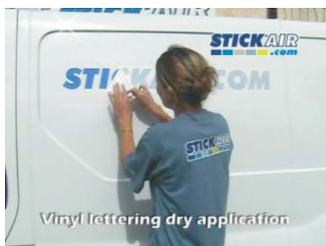
Vinyl lettering dry application You can now remove the application paper smoothing it flat. You will need to avoid pulling it towards you.
