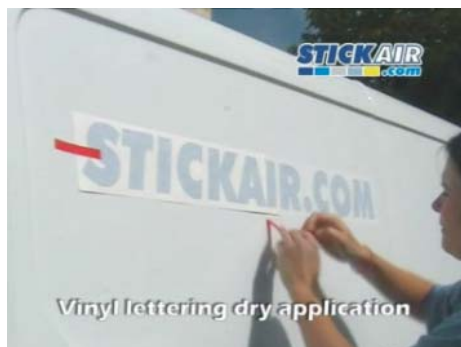
Vinyl lettering dry application Your lettering is now stuck down - you can remove the sticky tape.
