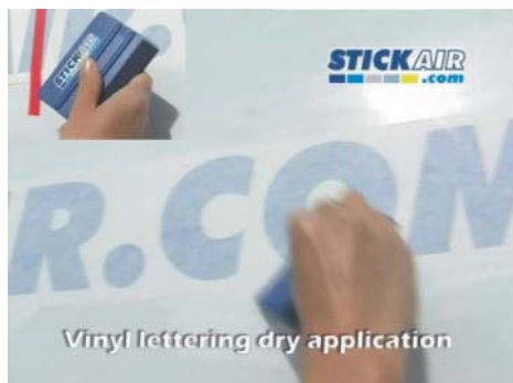
Vinyl lettering dry application Repeat the operation using the plastic side.
