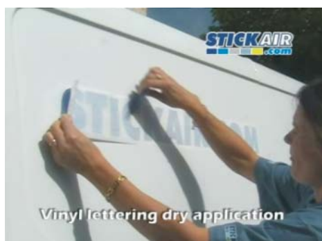
Vinyl lettering dry application Start the smoothing operations using the squeegee on the same side again.
