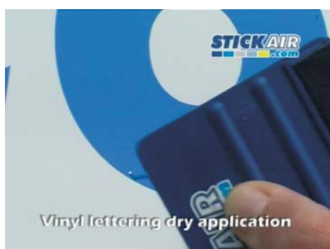
Vinyl lettering dry application If a bubble forms between the vinyl and the surface, remove it gently using the squeegee. If the bubble is too far from the edge of the letter, pop it with a needle.
