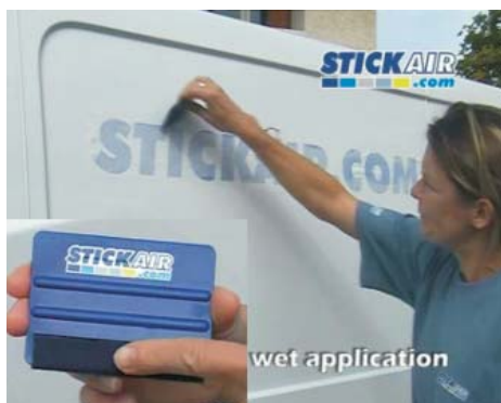
Use the soft part of the squeegee to remove the liquid. Ideally move from the centre to the outside.
