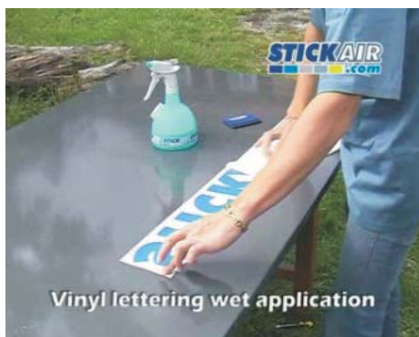
Remove the silicon-coated paper protecting the sticky part of the lettering.
